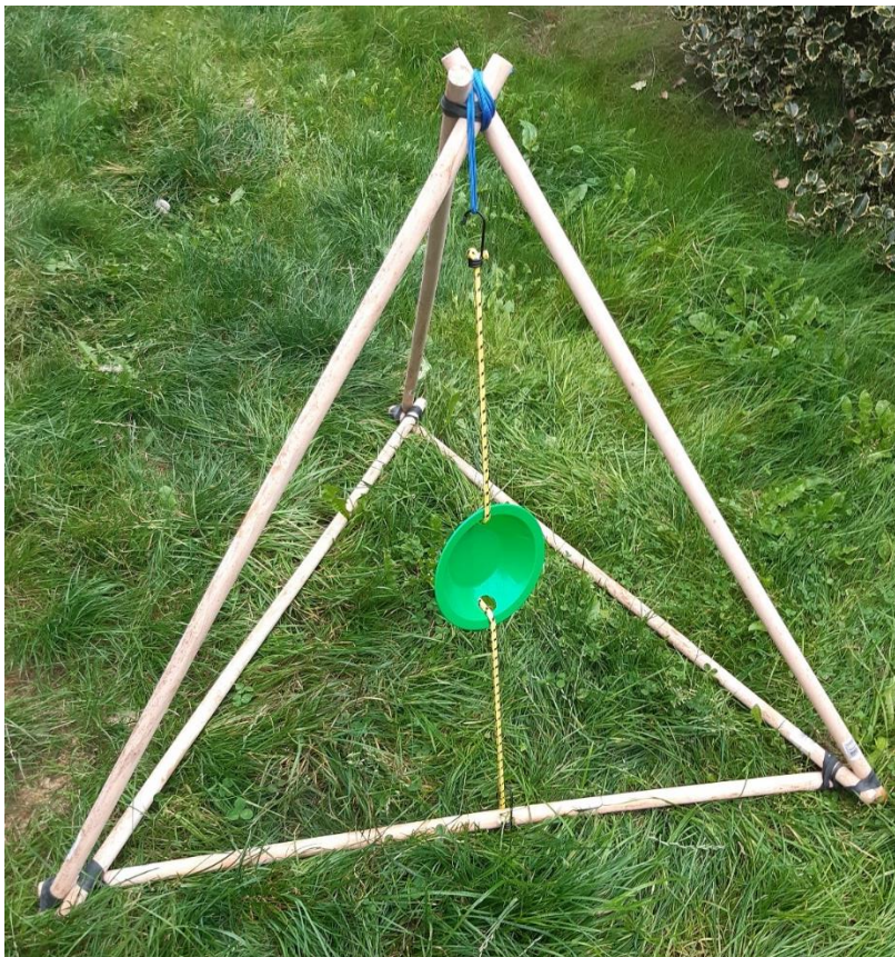
Simple Triangle frame with a bungee and catapult head fitted as a firing mechanism
